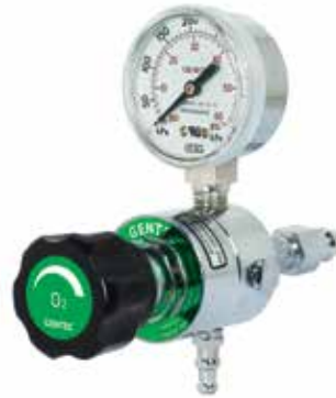
195MZ-O2-GS-HB4 Diaphragm-type regulator without flowmeter, with hose barb and GS inlet
